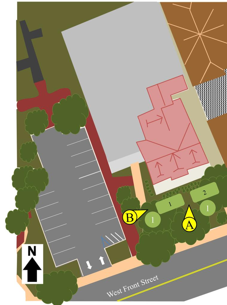
**1 BIORETENTION SYSTEM:** Rain gardens can be used to reduce sediment and nutrient loading to the Navesink River and increase groundwater recharge. Two rain gardens can be installed in front of the library to capture, treat, and infiltrate runoff from the downspouts in front of the building.
